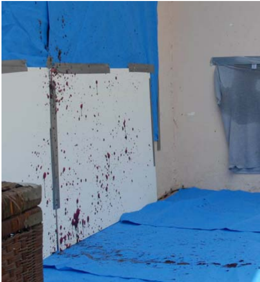
Figure 8. Impact spatter produced from blow struck in experiment 2.
