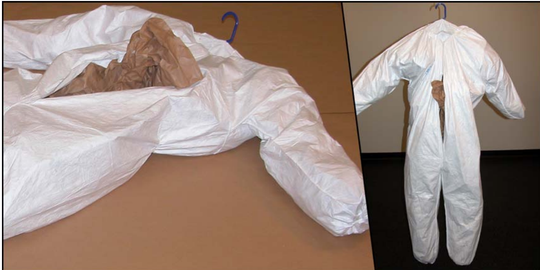
Figure 3. The overalls are then filled with paper filling and suspended via the coat hanger. Adjustments can be made to the stature of mannequin by the strategic use of adhesive tape.
