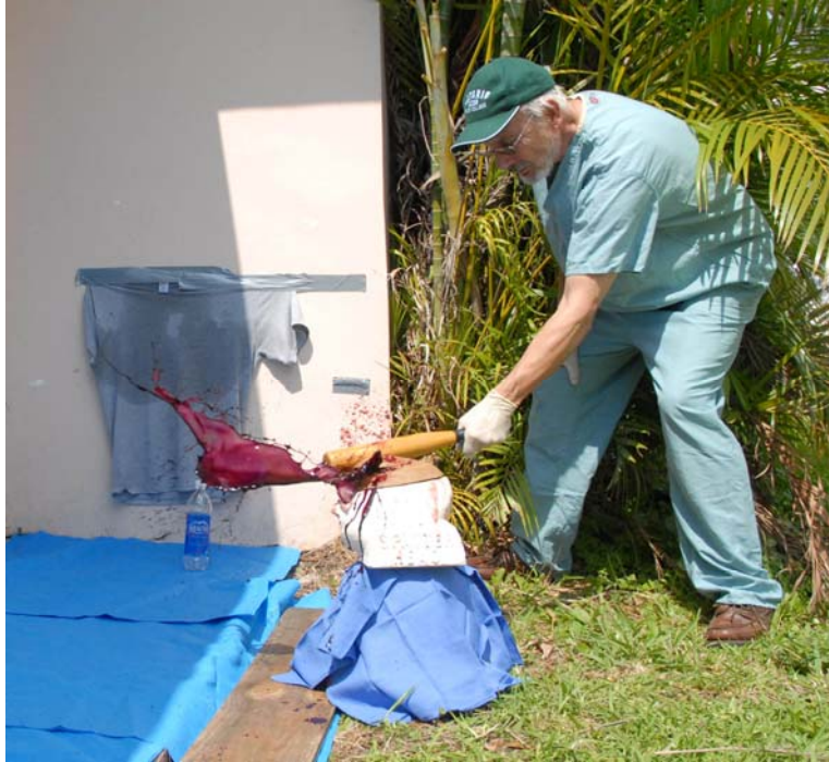
Figure 7. Impact of fish bat on Spatter Head showing expulsion of blood in experiment 2.
